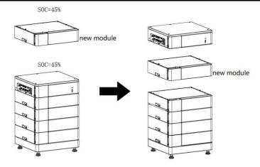
2. For battery modules with a long inventory time, charge the new module to 100% SOC with a charger (charge voltage is 56.16Vdc / 25A, cut off when current less than 2.5A), and charge the existing system to 100% SOC.
